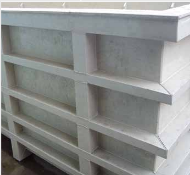
Electroplating tank, Turkey. Material: PP
